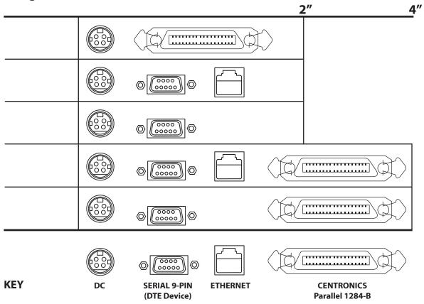
NOTE: Interfaces shown apply to Advantage LX printers with S/N's starting with "L"
