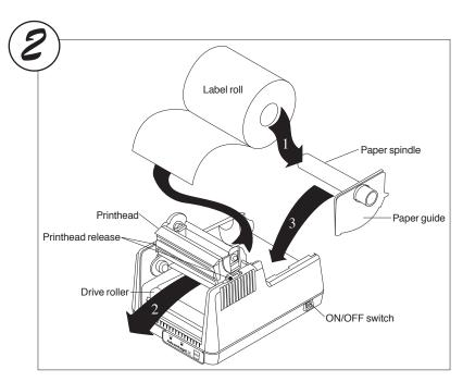
Thermal Transfer (TT) model shown. Printer is shown with media cover removed for clarity
