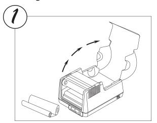
**NOTE:** Text on the ribbon leader should be face down in front of the printer.
