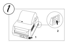
Press and hold the FEED button while turning printer ON
